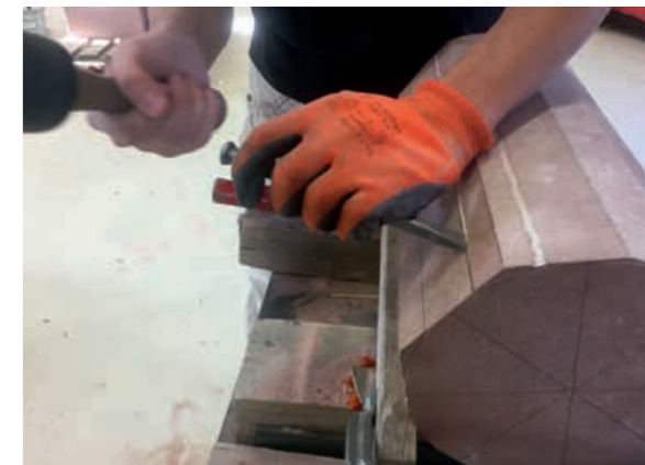
The cylindrical bollard is worked out of the cuboid shape in numerous working steps.
